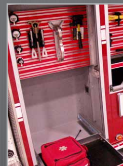
33" high of full-depth usable compartment space on split-depth body configurations
