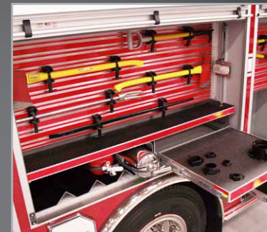
One (1) 26" w x 8" h x 25" d Drawer & Four (4) SCBA / Extinguisher Modules or (2) Four (4) SCBA for a Total of 8
