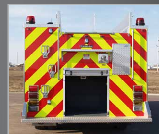
Large rear-center compartments for fans, rescue tools, booster reels, etc.
